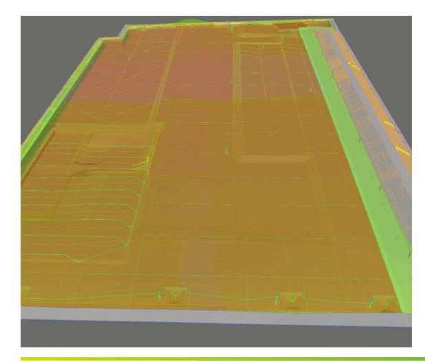
A combination BIM, CIVIL 3D, NAVIS WORKS and REVIT softwares were used to produce a full 3D model of the remediation system to include all the remediation elements including all Cap Type transition details, all pipeworks and their protrusions through the capping and integration details of the Capping system with Hydraulic Barrier.
